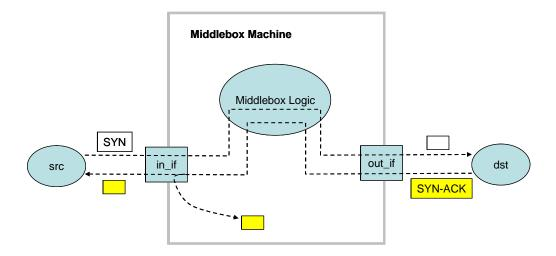
**Figure-6.5: Catching state creation.** Within a middlebox machine, a SYN or initial UDP message traverses the input interface ('in\_if'), IP layer and middlebox logic, and the output interface ('out\_if') in that order. Reply packets traverse in the opposite order. Reply packets are caught at the input interface to notice a state entry creation.
