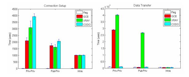
**Figure-7.2: UDP performance.** Each bar shows the average connection time of the corresponding middlebox traversal mechanism for each configuration. Error bars represent the standard deviation of the corresponding experiment.
