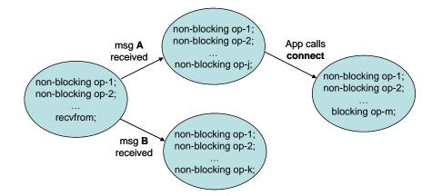
**Figure-6.2: State machine.** A socket moves from a state to another when the application calls a function for the socket or an event occurs. In this example, the state change from the leftmost state depends on the type of messages received (i.e. event type). On the other hand, the change from the top to the rightmost state is triggered by the application's connect call.
