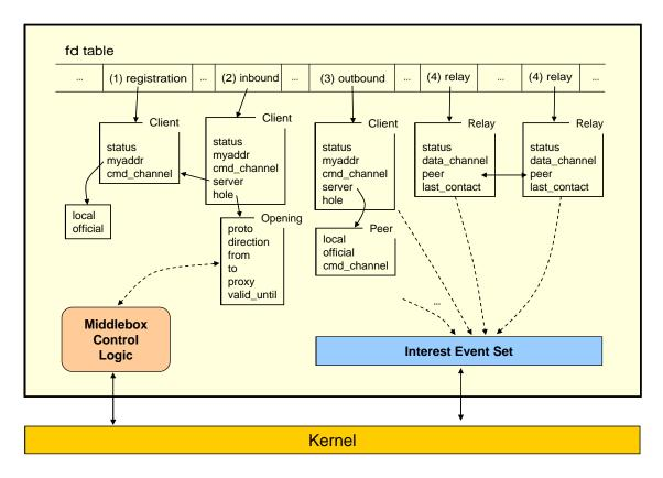
**Figure-6.4: Server structure.** Each transaction and relay point is represented by 'client' and 'relay' structures, respectively, which are linked from 'fd table'. Events of interest are dynamically collected into 'interest event set'. 'Middlebox control logic' interacts with Netfilter to add or delete rules to the kernel.
