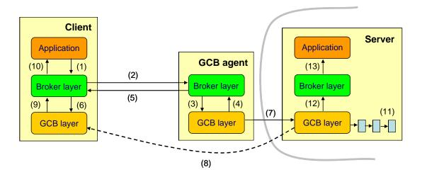
**Figure-5.2:** Public-to-private connection in GCB. GCB agent arranges a connection from a client in the public network to a server in the network it manages. Actual connection is made from the server to the client.
