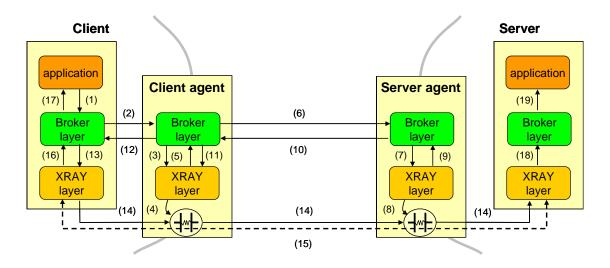
**Figure-5.4: Private-to-private connection in XRAY.** Both client and server agents create relay points to allow a connection from a client to a server in different networks.
