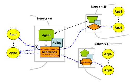
**Figure-4.1: Topology.** Each network may have one or more agents that control traffic into and out of it. In controlling traffic, each agent uses a traversal technique chosen by the network administrator.
