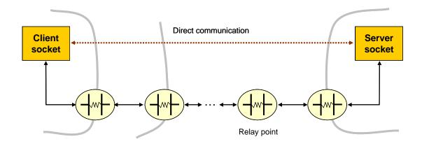
**Figure-5.3: XRAY basic idea**. XRAY creates on-demand end-to-end channels by placing relay points when direct communication between two points is impossible or undesirable.
