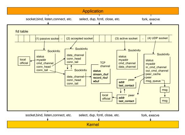
**Figure-6.1: Client structure.** Information ("SockInfo" in the figure) of each socket is linked from the file descriptor table ("fd table"). Auxiliary information of a socket is linked from its "SockInfo" structure.
