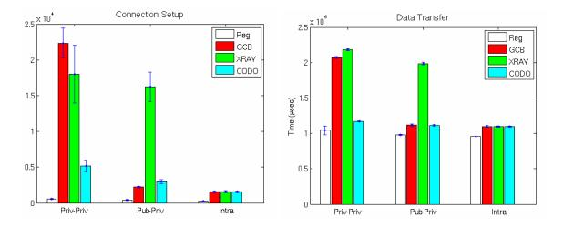
**Figure-7.1: TCP performance**. Each bar shows the average connection time of the corresponding middlebox traversal mechanism for each configuration. Error bars represent the standard deviation of the corresponding experiment.
