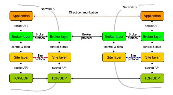
**Figure-4.2: Layered architecture.** The broker layer provides applications the abstraction of direct communication by coordinating difference between site protocols.
