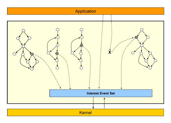
**Figure-6.3: Event handling.** Events of interest are collected from state machines of each socket. Gray circles represent the current states of state machines. The application may ask the client to add some event to the collection. However, some events may be translated into other events.
