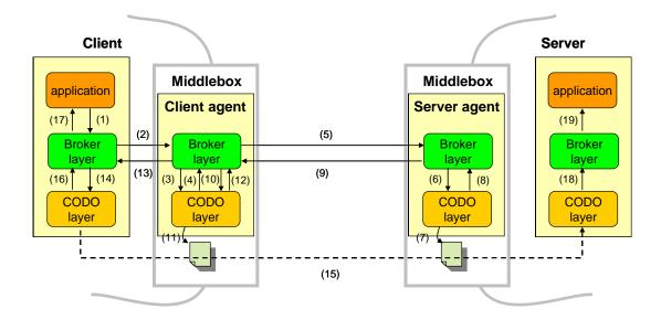
**Figure-5.5: Private-to-private connection in CODO.** Both client and server agents add rules to their middleboxes to allow a connection from a client to a server in different networks.
