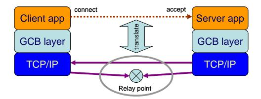
**Figure-5.1: GCB basic idea.** GCB decouples the direction of a connection from the role. It provides applications transparency by hiding the fact that connections may be made in the opposite direction or through relay points. The broker layer between the application and GCB layer is omitted for brevity.
