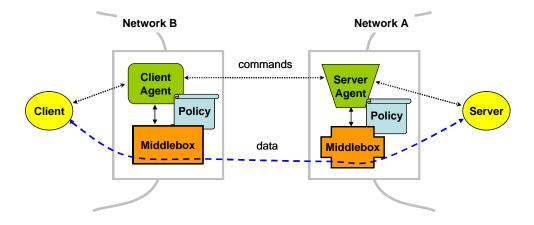
**Figure-4.3: Connection overview.** Applications (client and server in the figure) interact (dotted lines) with their local agents and then agents interact with each other on behalf of applications. Communication channels between applications (dashed line) are provisioned through cooperation between agents.
