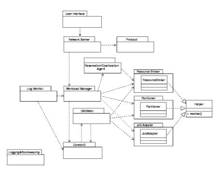
Figure 3: UML diagram describing the new DataGrid WP1 Workload Management System architecture.
